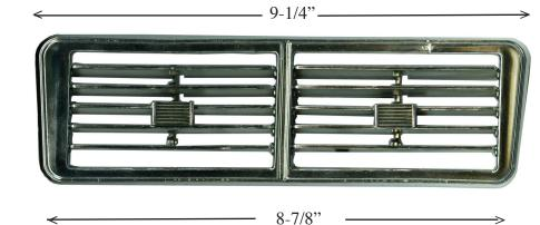
A couple of slats have uncoated spots on back edge. Viewable only if you shut the slats. That happend since the slats were closed during chroming. There is a repair on the right upper wall as shown in the picture.
