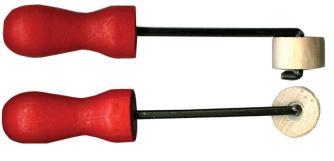
RO 101 \$4.95 1/2"O.D.x1/4"width Roller Wrap masking tape around the O.D. of the roller so you can reuse with different paint or vaseline on your next job. \*Purpose\* To prevent paint from sticking on raised letters or raised lip you want to stay Chrome (after painting dash the vaseline will wipe off). Or to letter white or black letters on rechrome plastic (use paint color of your choice).
